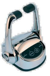
If the throttle fails, it may become unresponsive, causing the vessel to remain in gear with the propeller turning when neutral is desired, or preventing the engines from restarting. The potential throttle failures increase the risk of personal injury or property damage.
